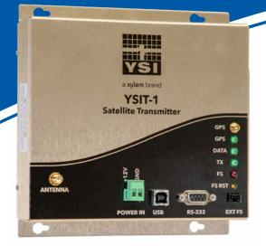
The **YSIT-1** is a secure and reliable GOES transmitter built for environmental data. Its operations are based on version 2.0 of the DCPRS certification standard. Sensor readings are transmitted over the GOES satellite system by linking to any Storm 3 or XL Series Data Logger. The YSIT-1 is ideal for Surface Water Data Collection Platforms, Meteorological Stations, and Water Quality Measurement Stations.
